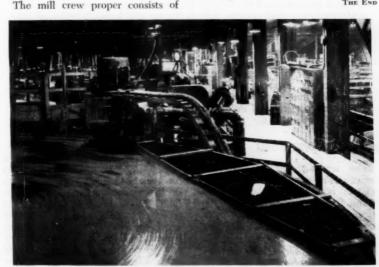
CCD CIRCUIT consists of four 60-by 12-foot Dorr thickeners; using Separan, underflow densities of 60 percent have been maintained; load is usually controlled by adjusting speed rather than stroke of diaphragm pumps handling underflows.
